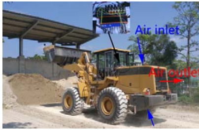
Fig. 6. Air flow direction and data acquisition instrument
